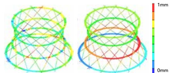
**Displacement in a hyperboloid reef due to vertical (left) and horizontal (right) forces.**
